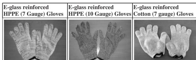
Figure 1 : Photographs of High performance knitted E-glass reinforced HPPE and Cotton gloves
